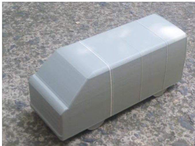
Figure 4. 2. The prototype of Toyota HiAce midi bus for wind tunnel test.
