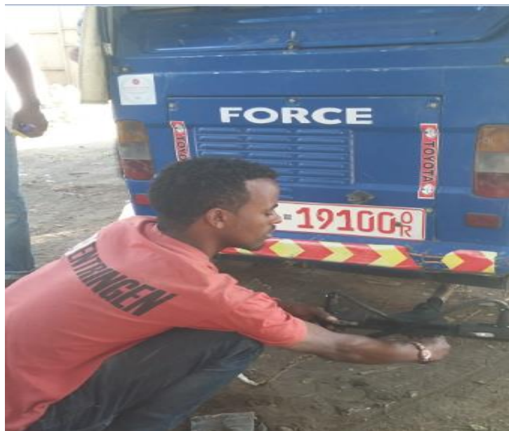
Figure 12: Inserting opacity probe to vehicle tailpipe
