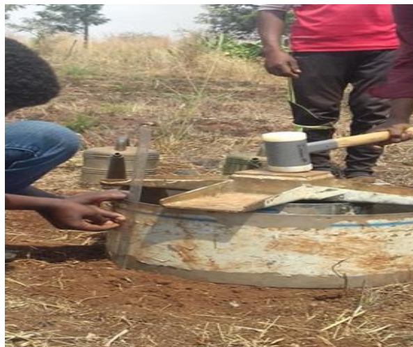
Figure 3. 7 Double ring infiltrrometer instalation
