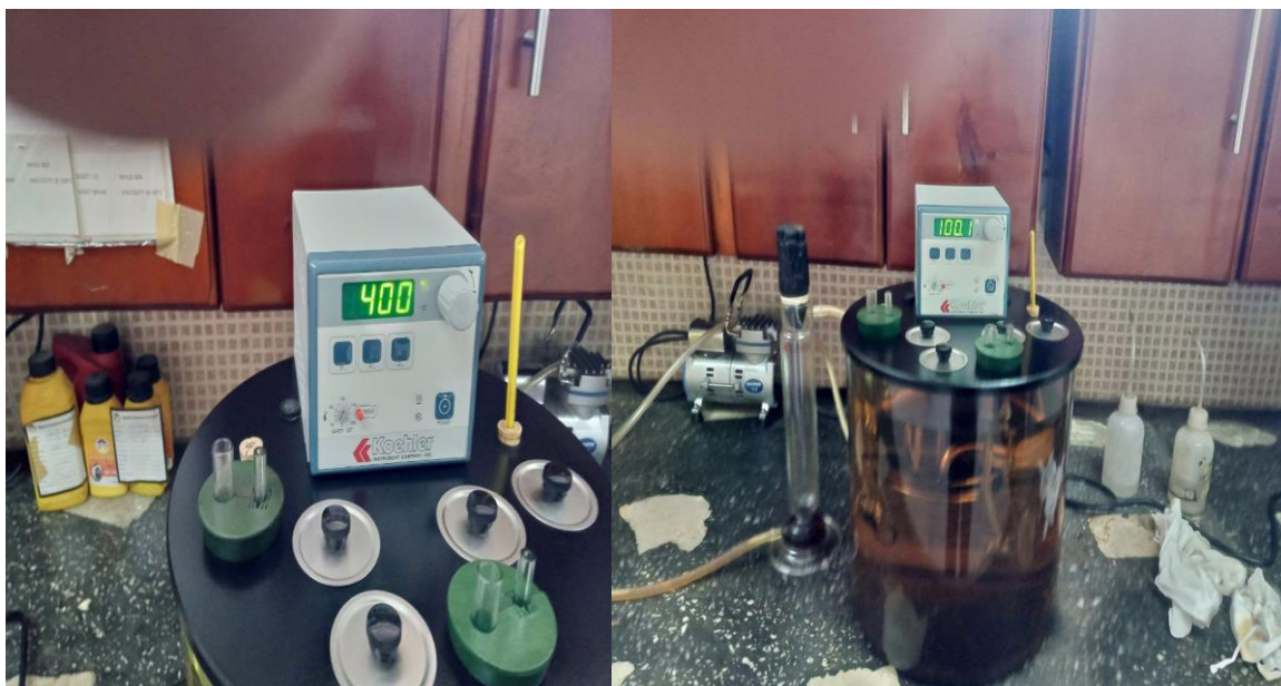
A. Calibrated viscometer at 40 °C
