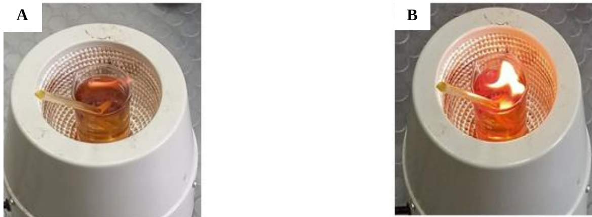
Figure 3.7. Flash point and Fire point determination test (A. Flash, B. Fire point)
