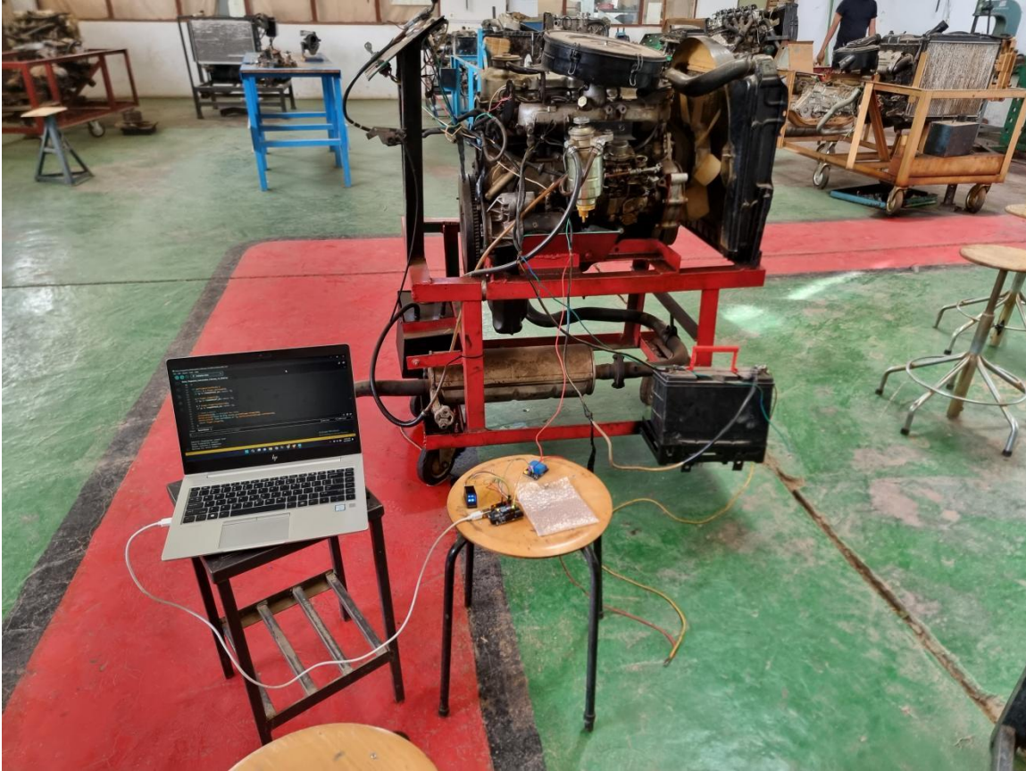
Figure 4. 12 Fingerprint authentication based engine starting on Nissan diesel TD27
