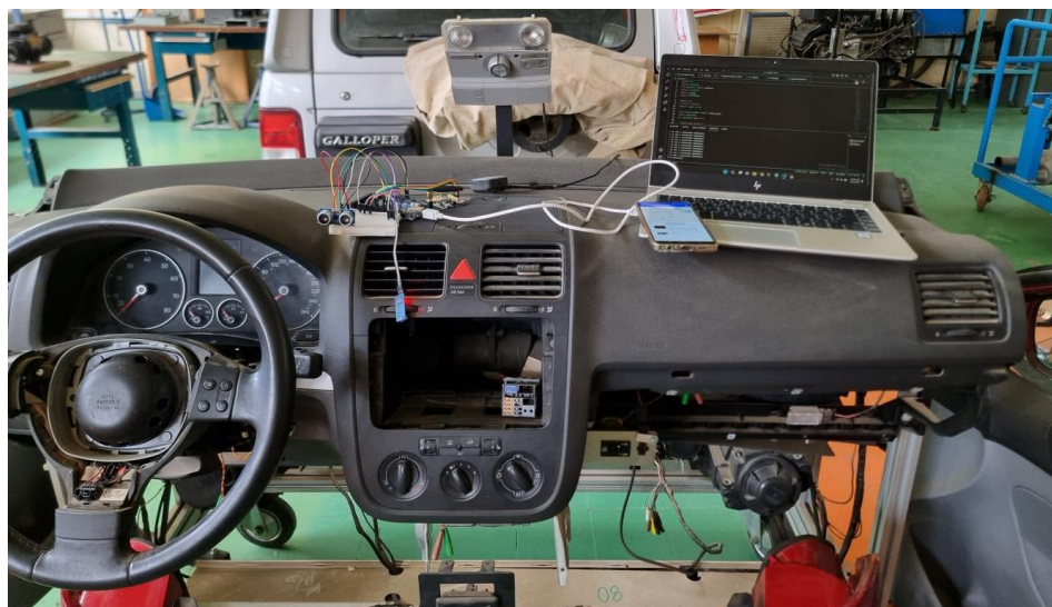
Figure 4. 18 Implementation of the theft deterrence system
