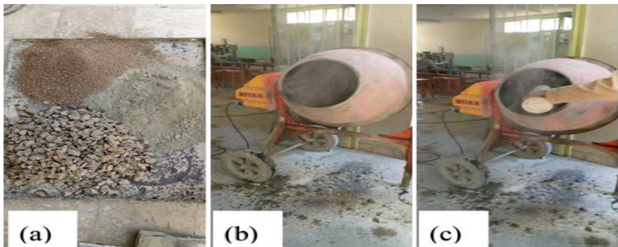
Figure 3.8: Batching and mixing procedures: Batched ingredients (a), dry mixing (b) and wet mixing (c)
