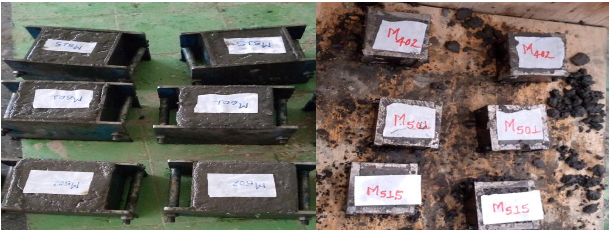
Appendix E3: Captured pictures of Casted Concrete Samples: (150*150*150) mm sized cube for compressive strength test and (70*70*70) mm sized cube for water absorption test.
