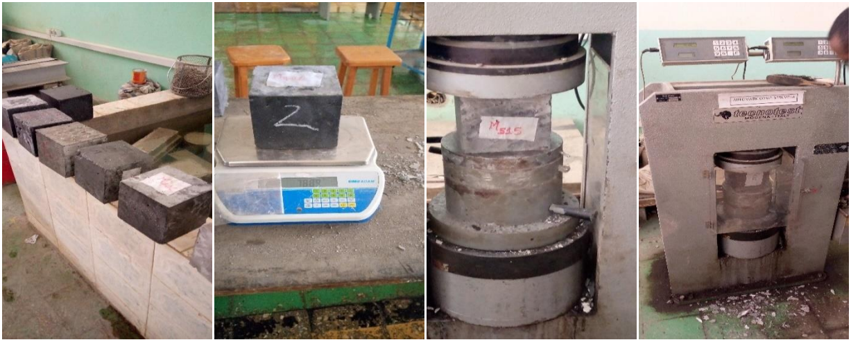
Appendix E5: Pictures taken during sample preparation for compressive strength test and During conducting the test.
