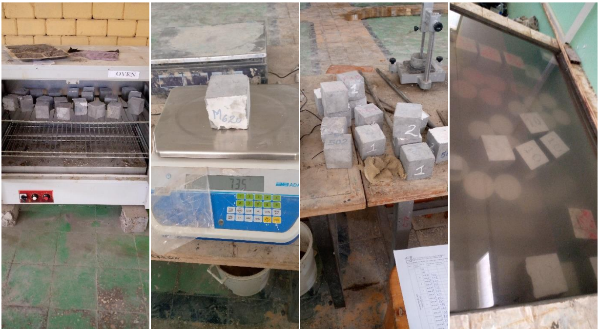
Appendix E6: Pictures taken during oven drying, weighing and submerging samples in . Water for water absorption test.
