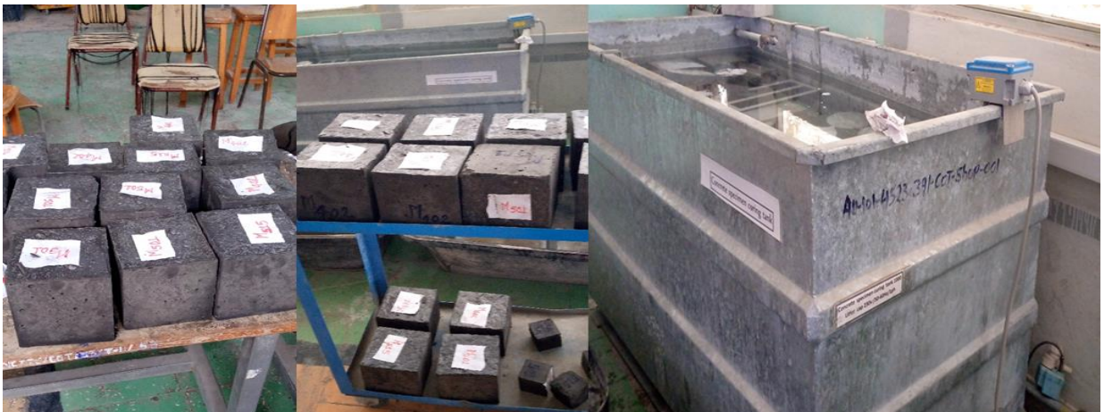
Appendix E3: Captured pictures of Casted Concrete Samples: (150*150*150) mm sized cube for compressive strength test and (70*70*70) mm sized cube for water absorption test.
