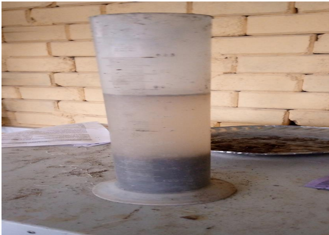
Figure 3.3: Sand Silt Content Test
