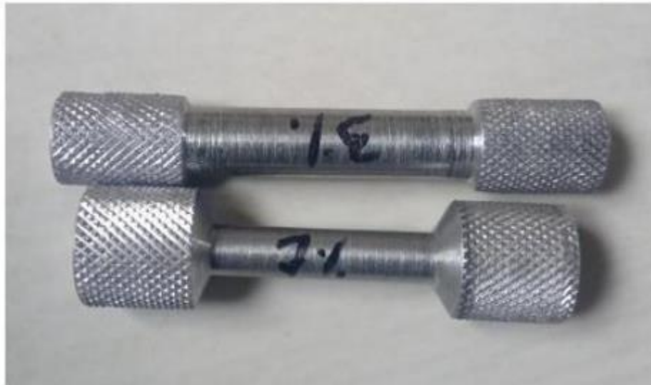
Figure 2. 2 Tensile test specimens ( Hosamani et al, 2016 )
