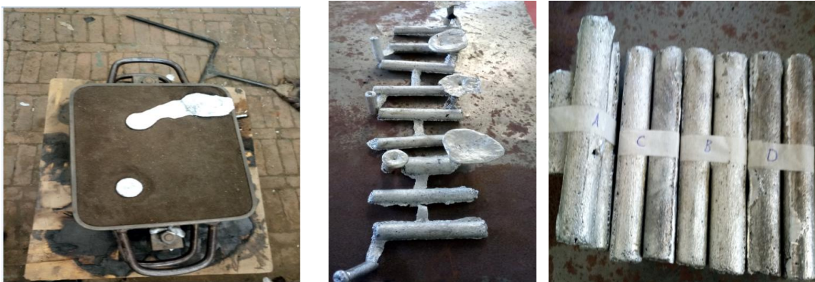
Figure 3. 2 Specimen fabrication by stir casting process
