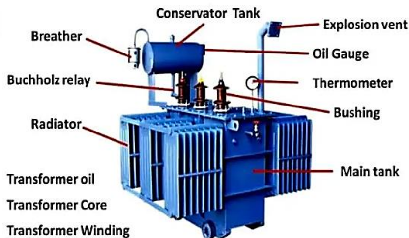
Figure 2.1 Parts of power transformer
