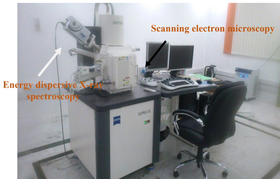
Figure 23: Photo view of CARLZEISS high resolution microscope with Oxford instrument Energy Dispersive X-ray Spectroscopy (EDS) is utilized to analyze elemental composition analyses of the nanoclay by using the Oxford instrument with five iteration of each sample.
