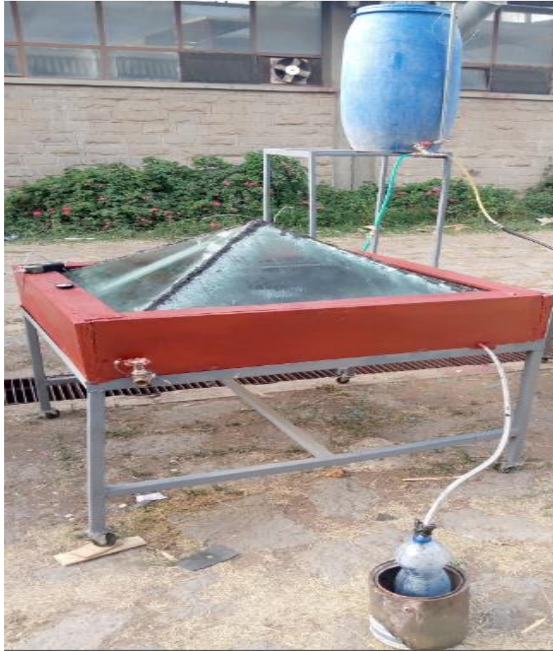
Figure 5.6: Experimental setup of the modified pyramid solar still
