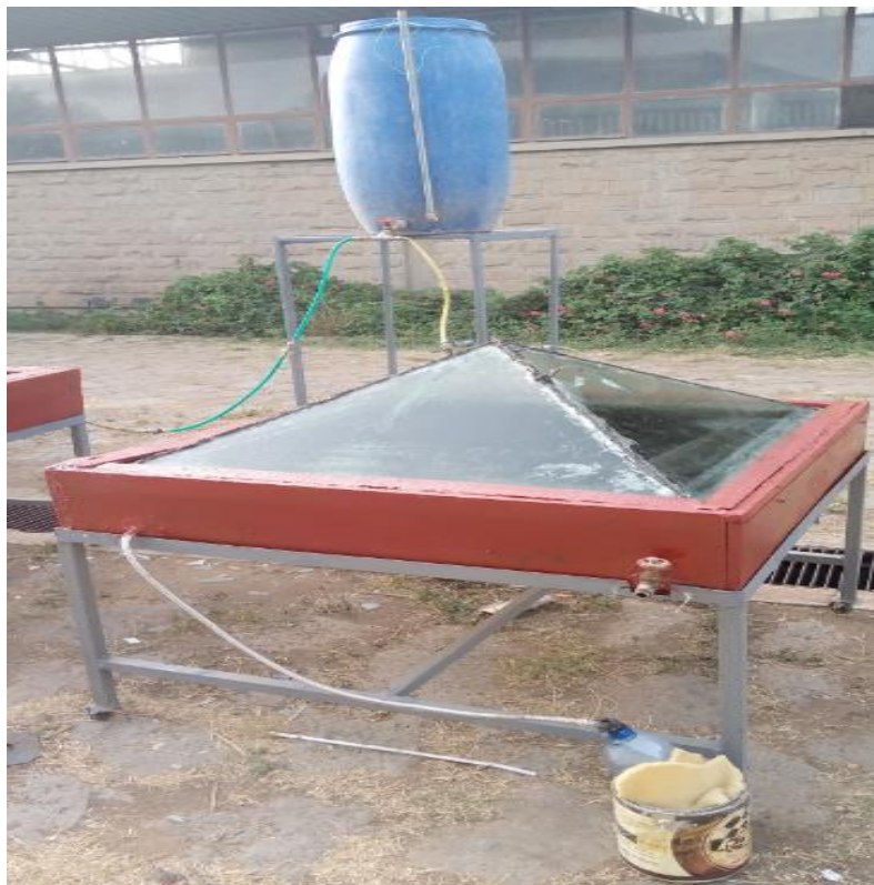
Figure 5.3: Experimental setup of the conventional pyramid solar still
