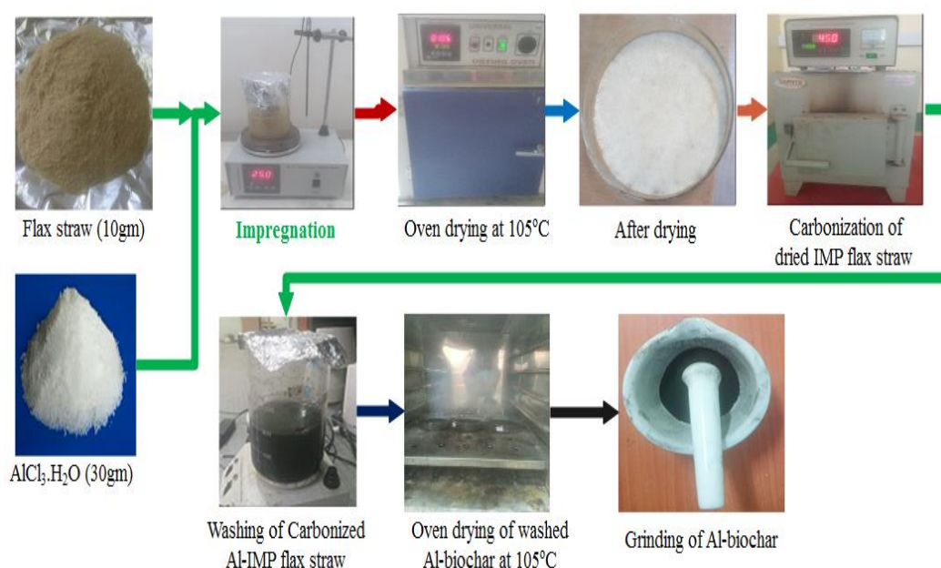
Figure 3. 3. Preparation of Al-bio char
