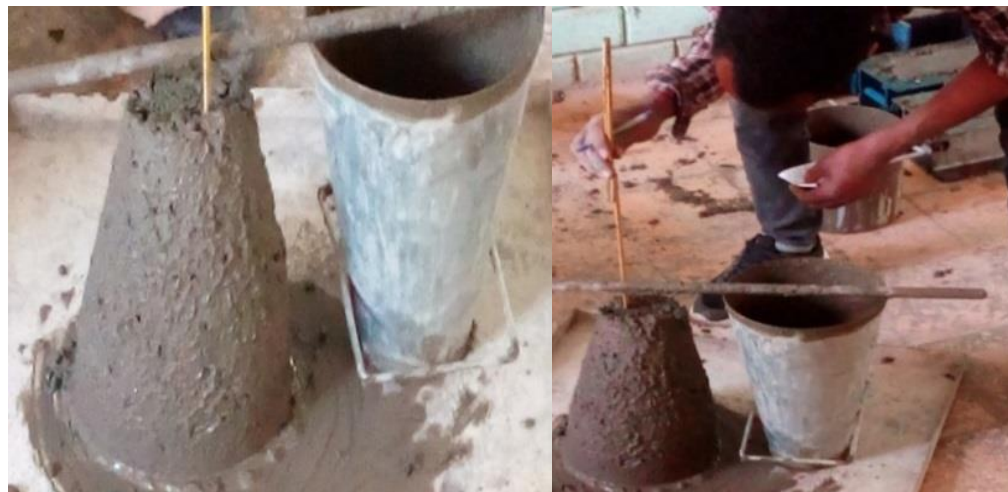
Figure 4.4 checked Concrete slumps
