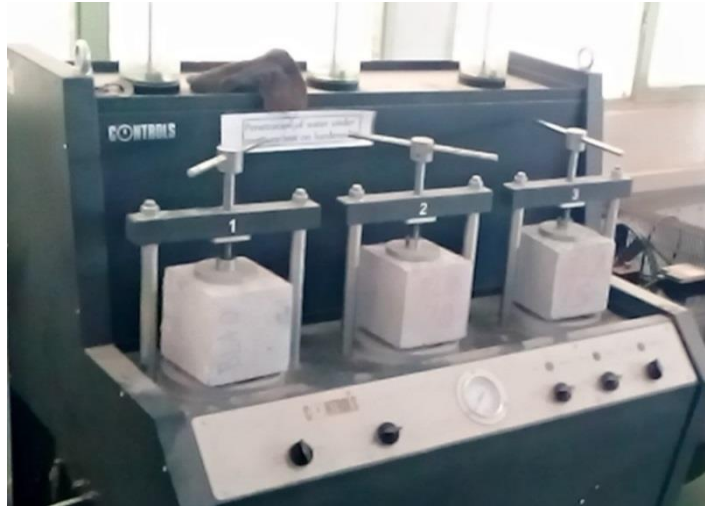
Figure 4.10 Specimens Ready for Water Permeability Test
