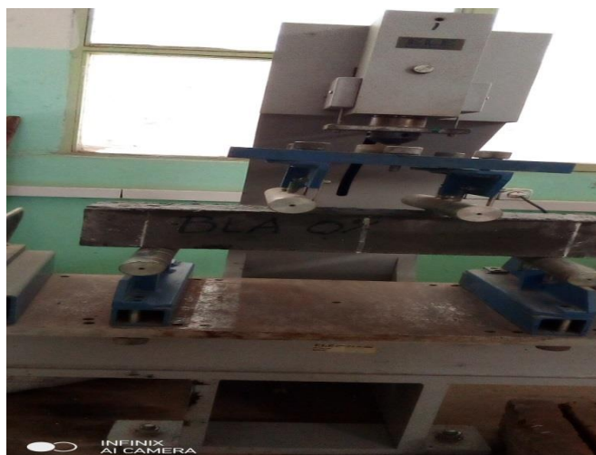
Figure 4.7 Flexural Strength of Concrete Is Being Tested
