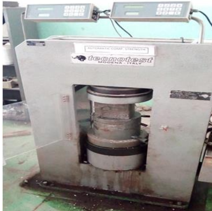
Figure 4.5 Compressive Strength of Concrete Is Being Tested
