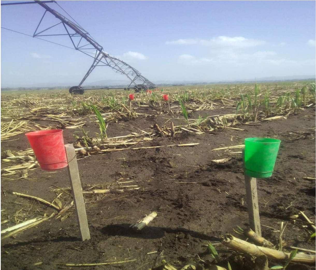
Figure 3.2 Catch can alignment during test
