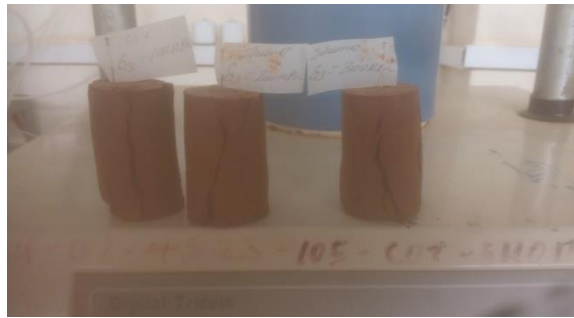
Samples after shear failure
