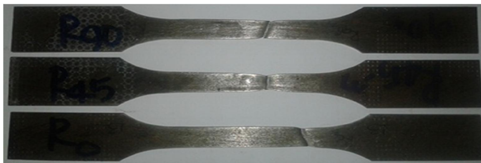
Figure 4.3 EN-10149-2 steel sheet metal Specimen after Tensile Test
