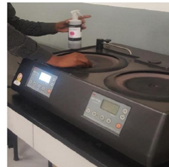
Figure 3.4 Rotating silicon carbide paper with diamond suspension
