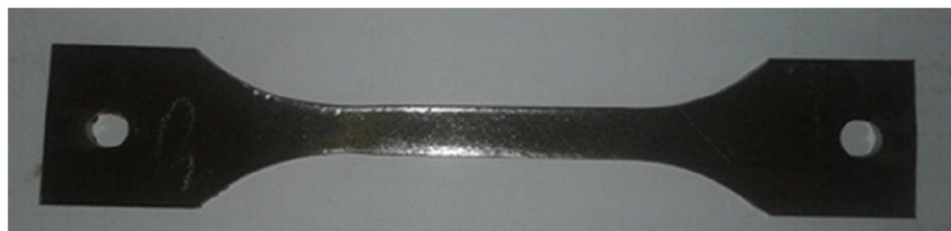
Figure 3. 14 Typical Specimen for plastic strain ratio test
