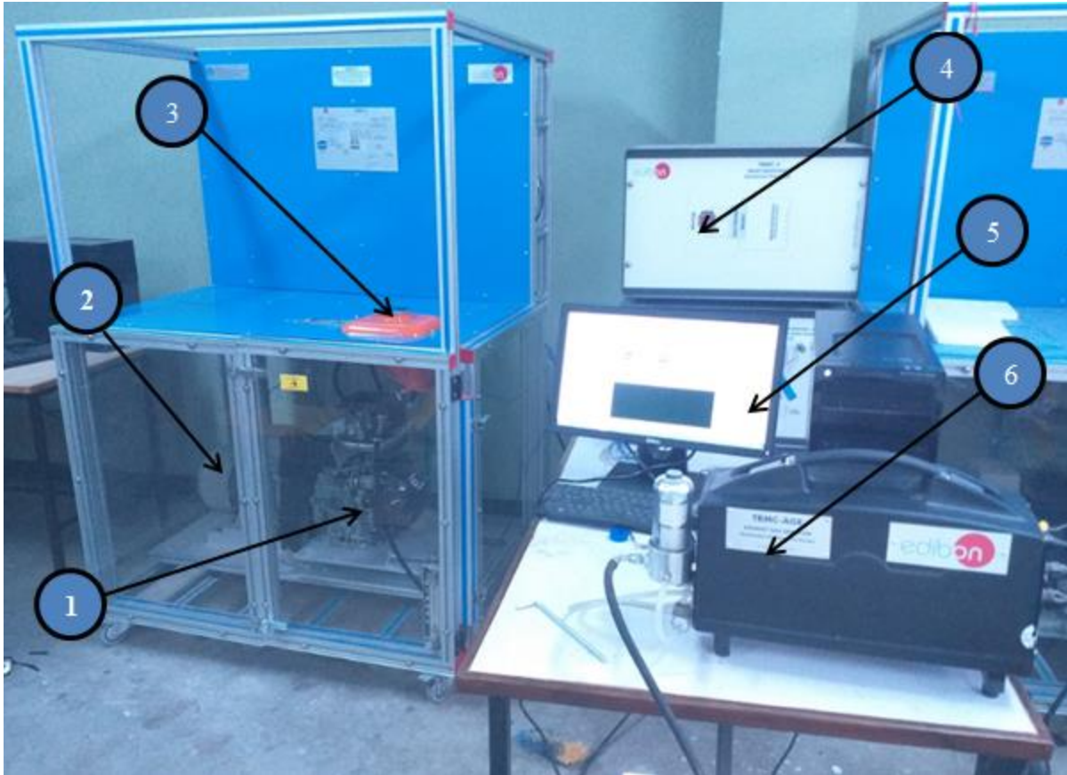
1 Diesel engine, 2 Asynchronous motor, 3 fuel tank, 4 SCADA control system, 5 Computer, 6 Exhaust gas analyzer
