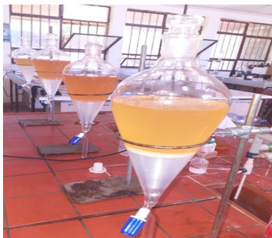
Figure3.14 Third and fourth stage of washing COME
