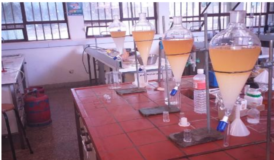
Figur3.12 First stage of washing of COME
