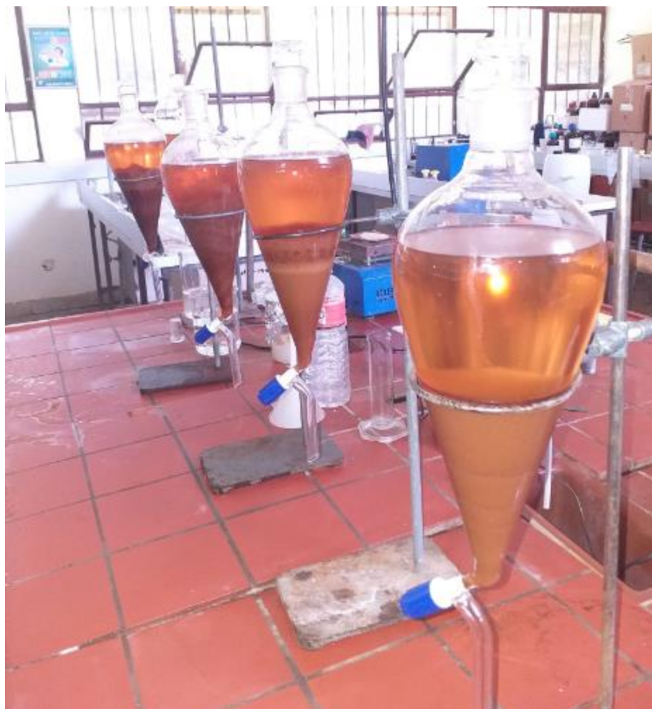
Figure3.11 After separation of glycerol and soap from COME
