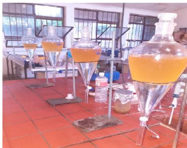
Figure3.14 Third and fourth stage of washing COME
