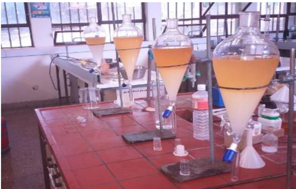
Figure3.13 Second washing step of COME
