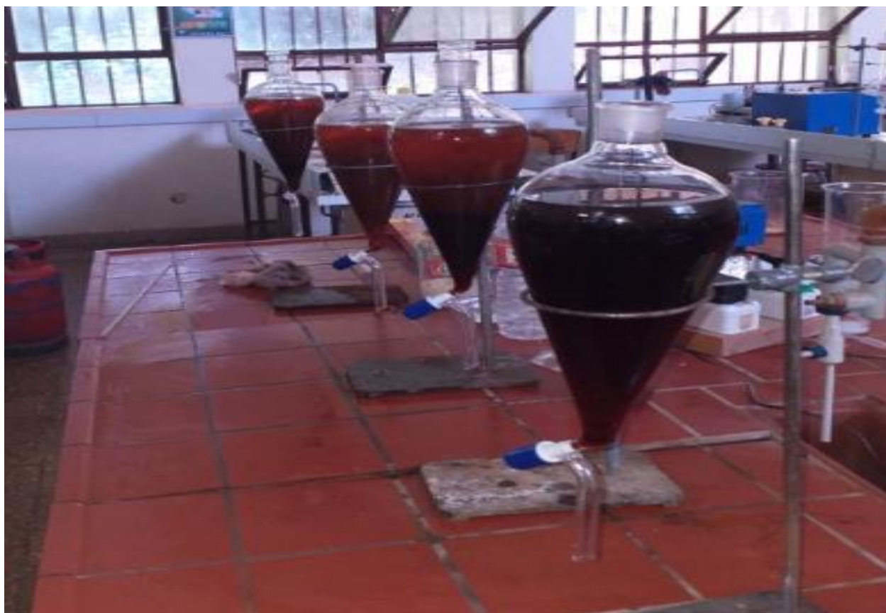
Figure3.10 Before separation of glycerol and FAME
