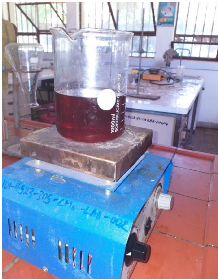
Figure 3.7 Preheating of cotton seed oil
