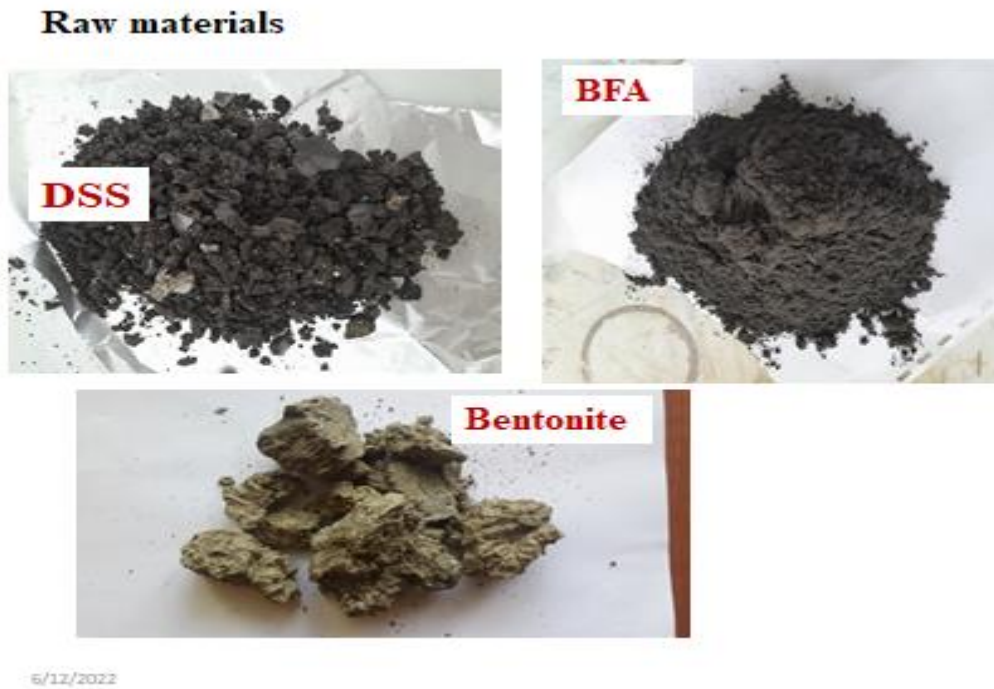
Figure. 7.1. Raw materials used for preparation of ceramsite.
