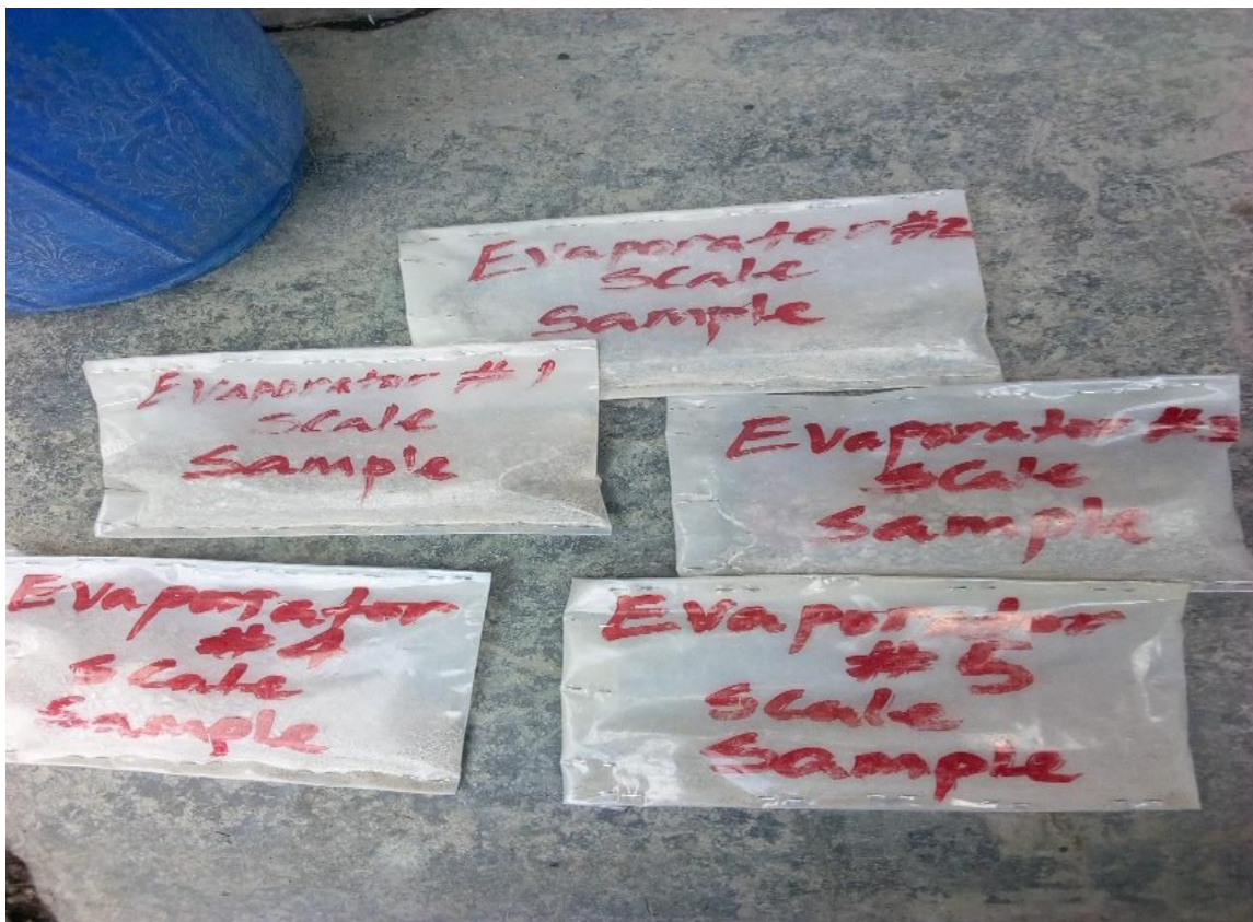
Appendix Figure 2 Collected scale samples from new WSSF multiple effect evaporators
