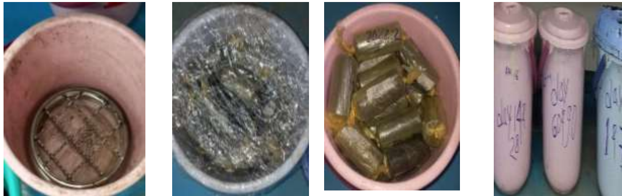
Figure 3.12 The process of method to cure and testing UCS test
