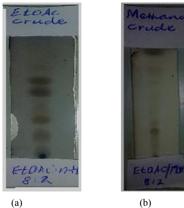
Figure 5: TLC profile of the EtOAc (a) and MeOH (b) extract.
