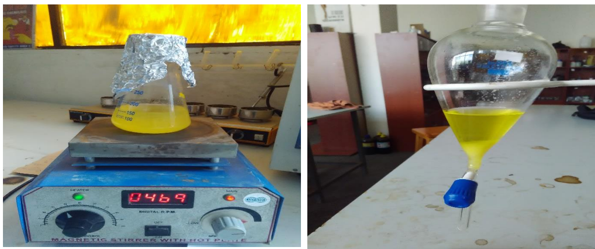
Figure 7: Stirring the blend with magnetic stirrer and separating with separator funnel
