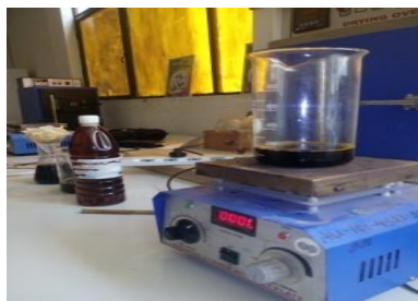
Figure.3.2 Heating of cottonseed oil on magnetic stirrer hot plate
