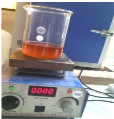
Figure.3.5 Heating and drying the biodiesel
