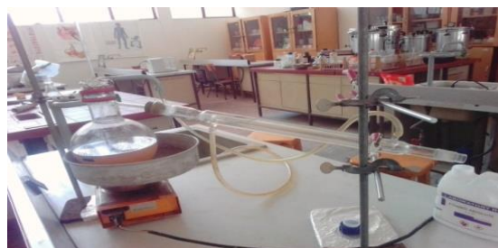
set up of simple distillation of ethanol alcohol
