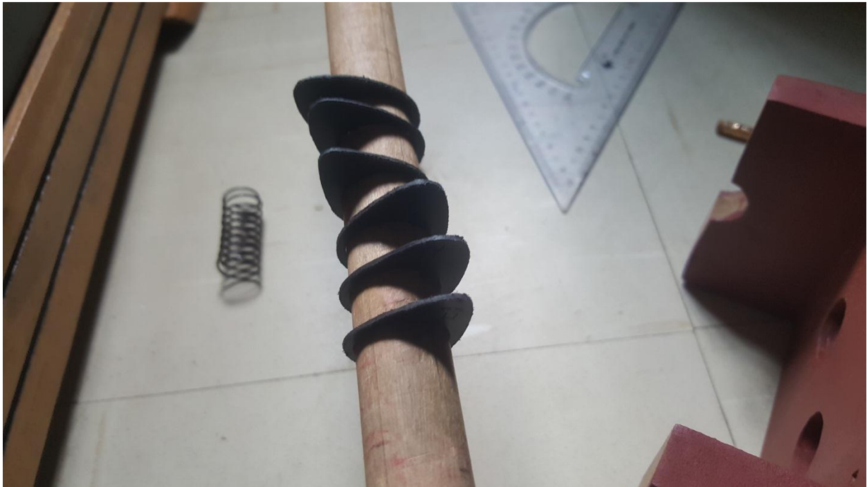
Appendix B3 Cam profiles arranged on a wooden shaft
