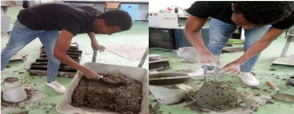
Figure 3:4 slump test of concrete (laboratory photo)
