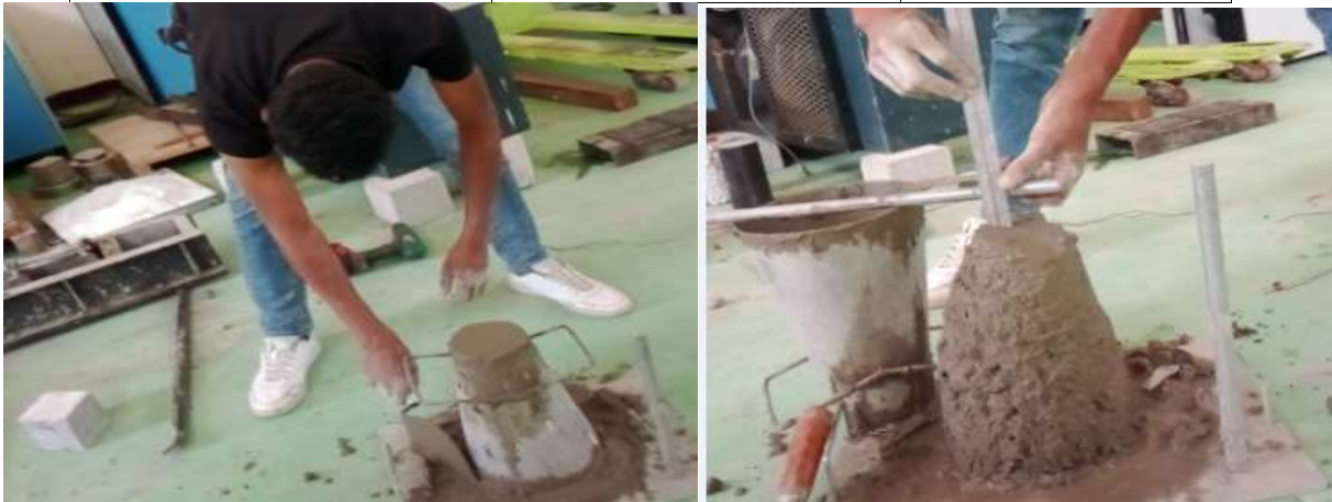
Figure 5:4 slump of concrete
