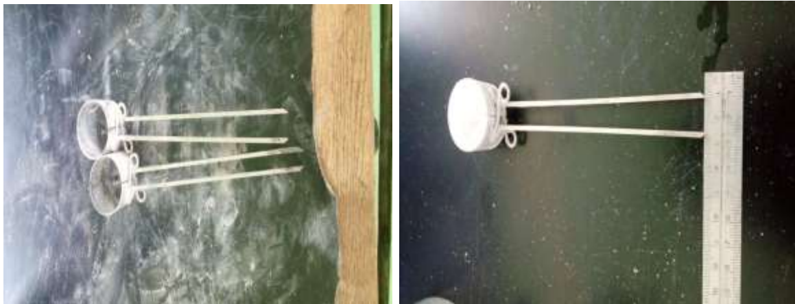
Figure 4:2 'Le Chatelier' apparatus (Lab photo)
