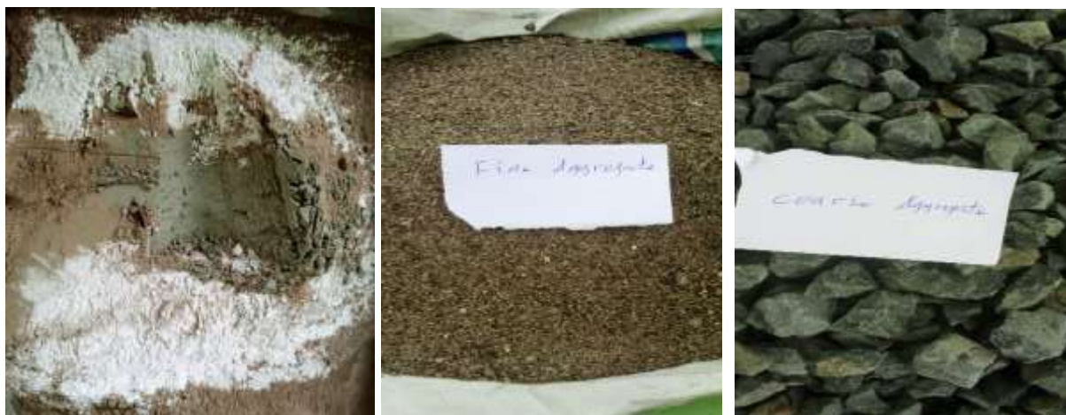
Figure 3:3 Proportion of materials for concrete specimens of concrete (laboratory materials).
