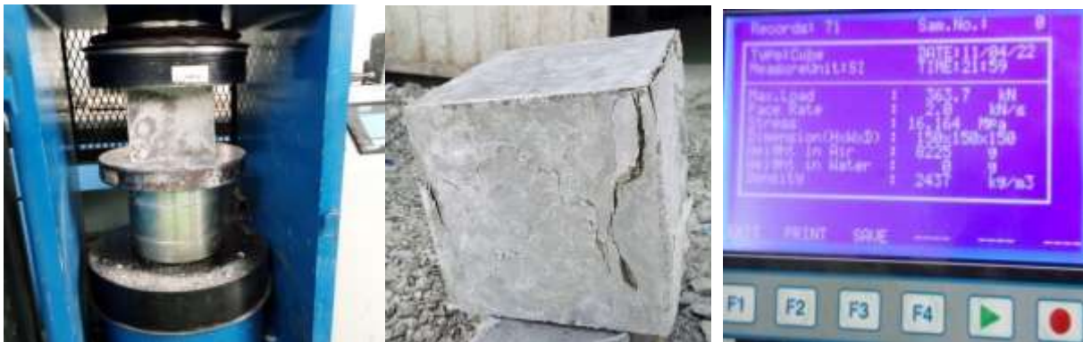
Figure 3:6 Compressive Strength of the Concrete (Laboratory photo).
