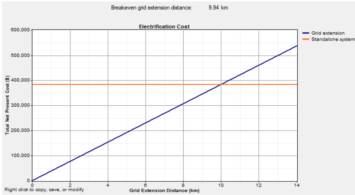
Figure4. 6 Breakeven grid extension distance obtained using HOMER
