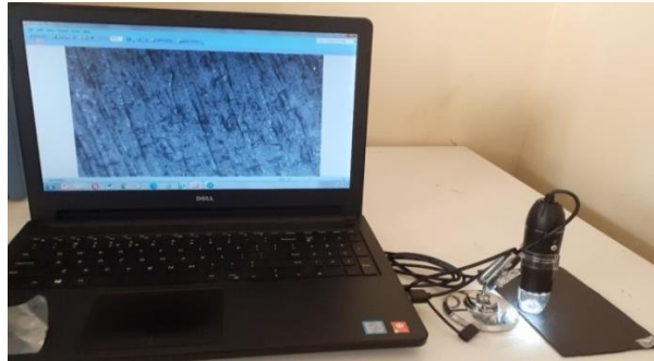
Figure 4. 17: Image of polished leather sample taken by digital microscope
