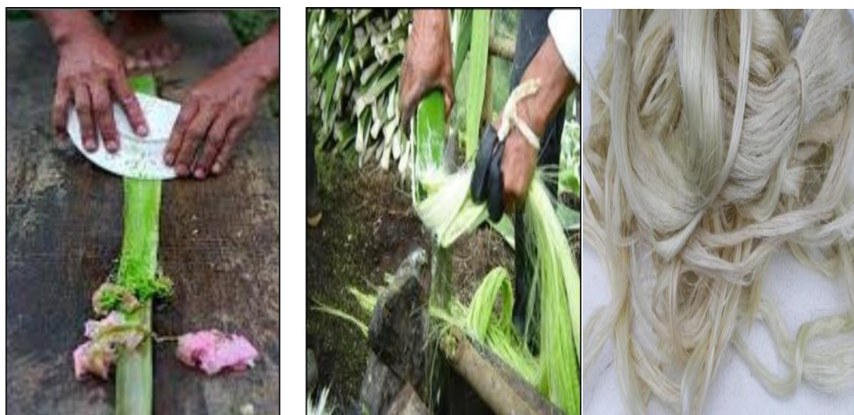
Figure 2.9 Sisal fiber extraction process ( Serration process) &Extracted Sisal fiber [36]
