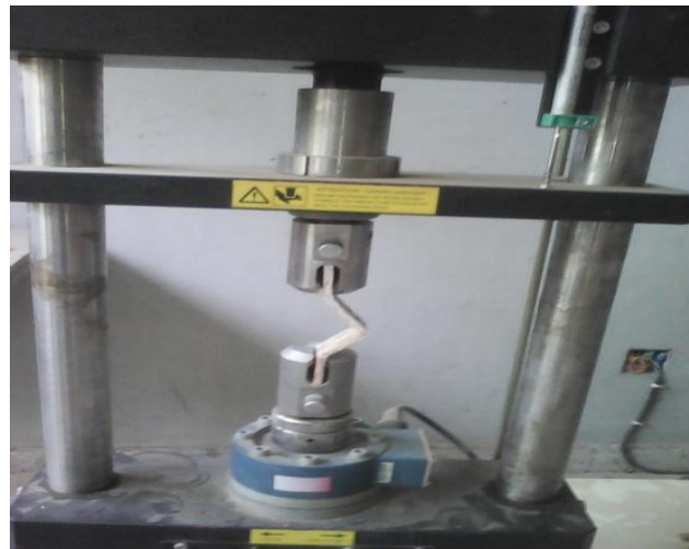
Figure 3.31 a. SFRUPRC specimen for Compression Test b. Specimen Under Compressive load c. Specimen breakdown under compression loading.
