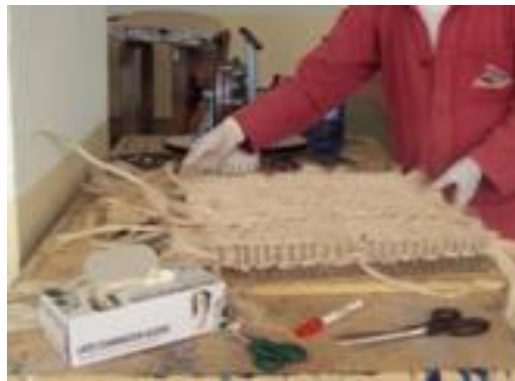
Figure 3.15 Arranging the fiber using weaving (loom) equipment
