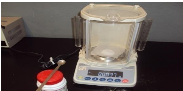
Figure 3.9 Weight measuring of Sodium hydroxide Utilizing Analytical Precision Balance
