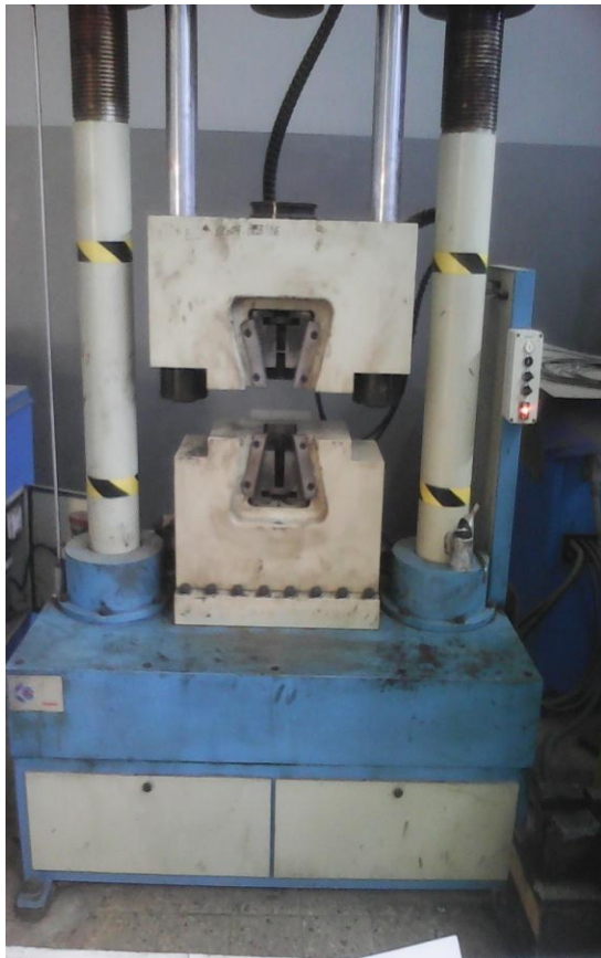
Figure 3.27 Universal testing machine (UTM) Material Testing System in Ethiopian Conformity Assessment(ECAF) Mechanical Testing laboratory
