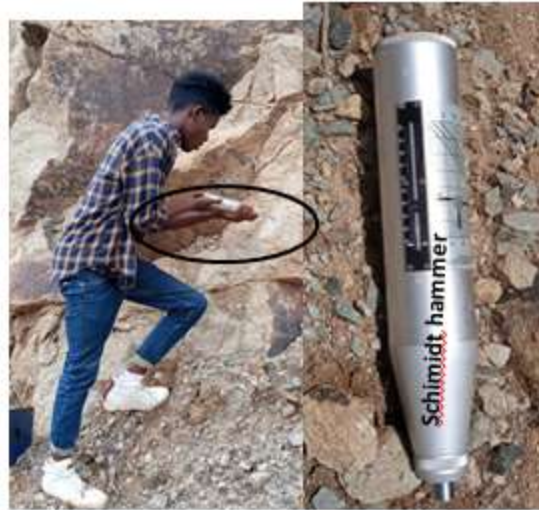
Figure1.22 Conducting Schmidt hammer test on ignimbrite, the northern part of town at the quarry site
