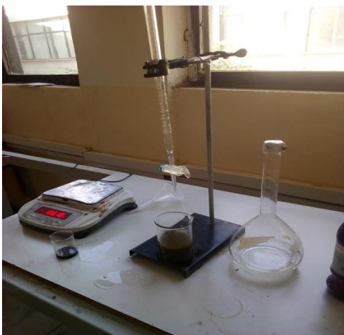
Figure: Total acid value determination
