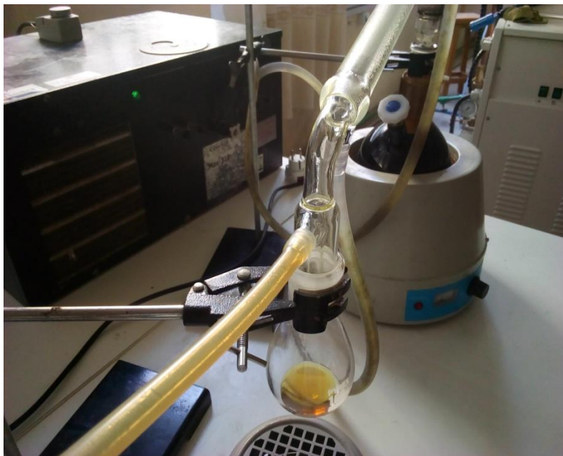
Figure 4.8 Light fuel (diesel) recovery
