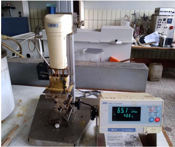
Dynamic viscosity determination
