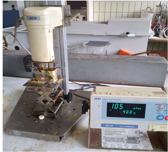
Dynamic viscosity determination
