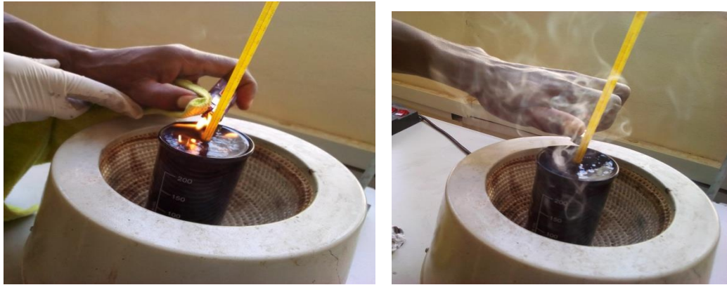
Figure: Flash point determination
