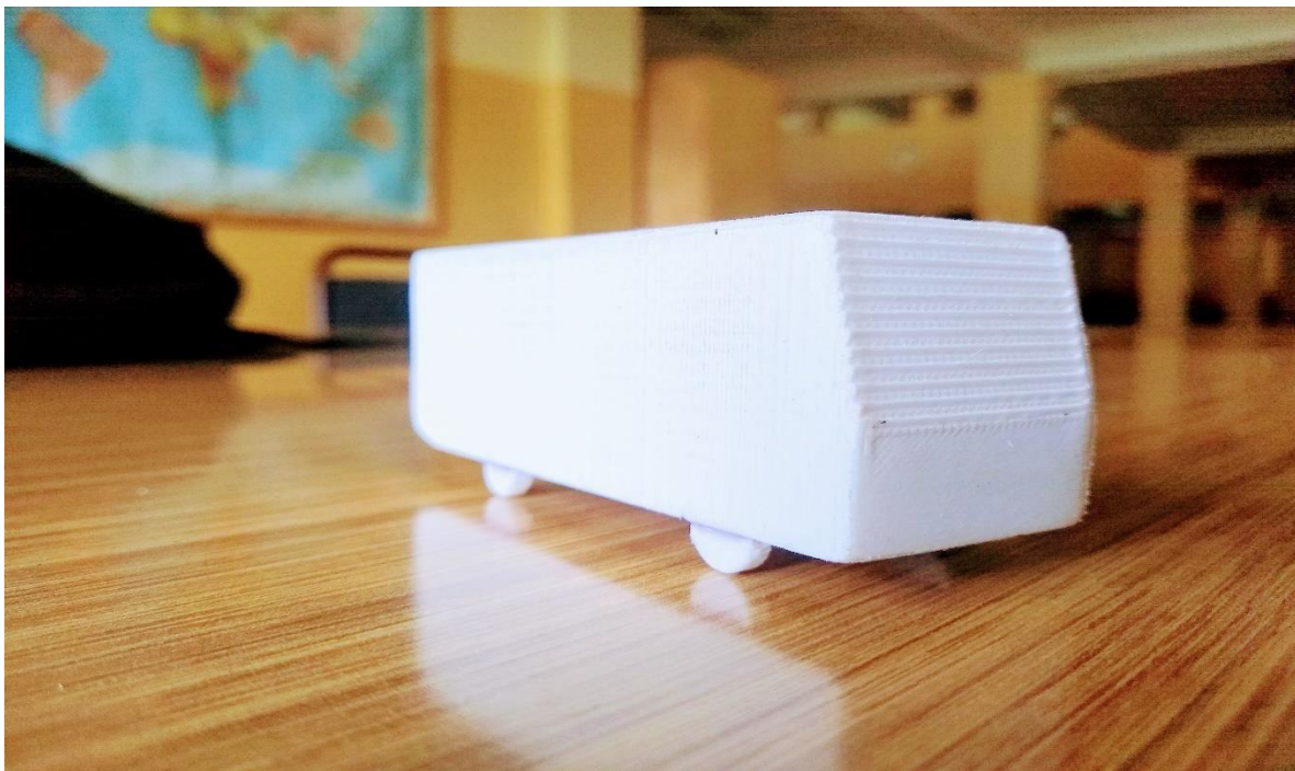
Figure 4. 2: The prototype of Isuzu midi bus for wind tunnel test
