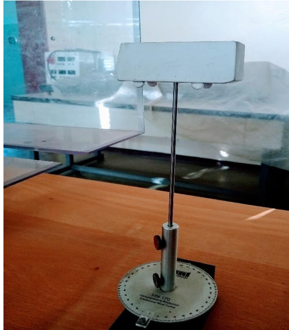
Figure 4. 5: Securing the prototype of Isuzu midi bus in the wind tunnel
