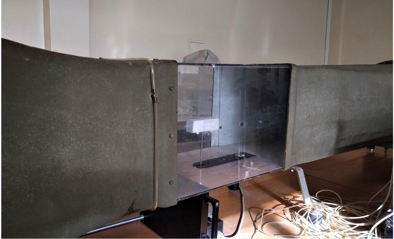
Figure 4. 7: Prototype of Isuzu midi bus mounted in the wind-tunnel
