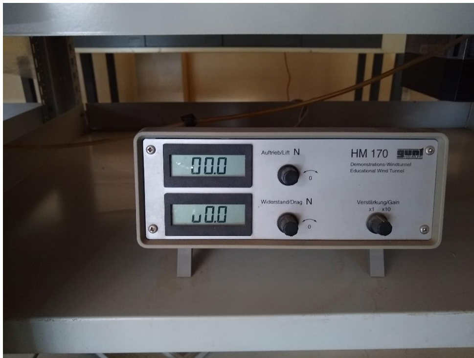
Figure 4. 6: Zeroing the measuring equipment
