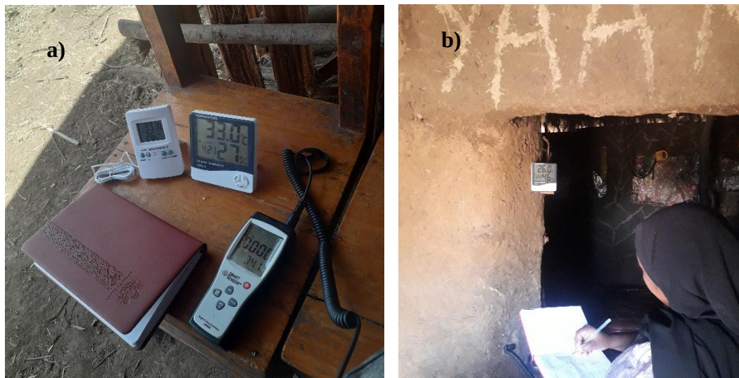
Figure 3.4: a) outdoor environmental measurement under verandah and used for cross checking the instrument reading b) indoor temperature measurement by the author
