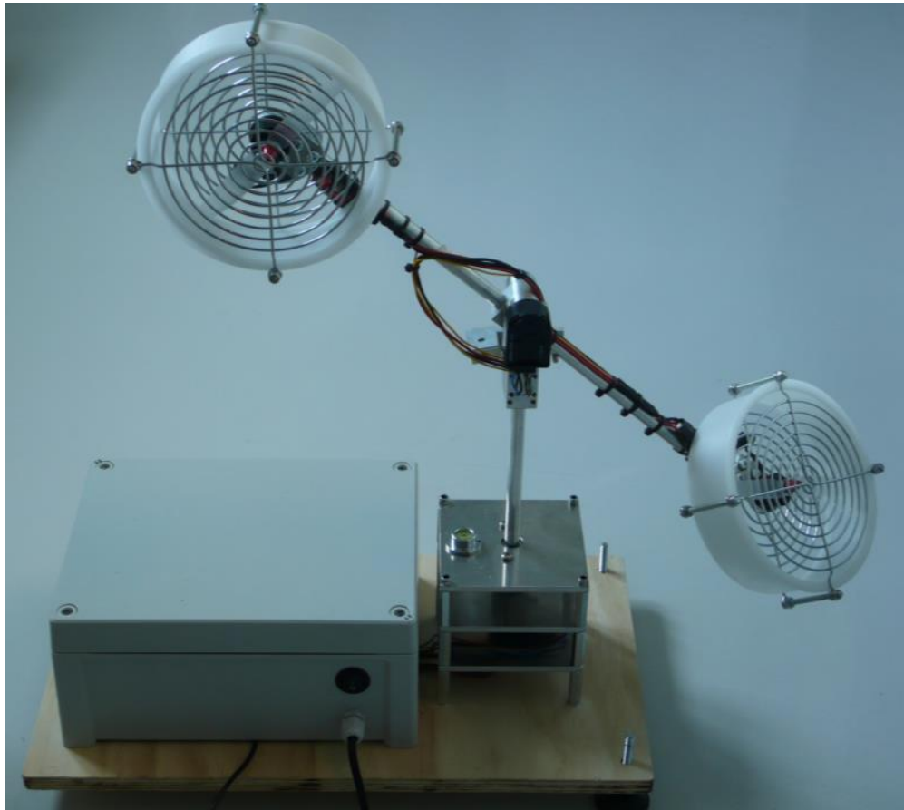
Figure 2-1 An image of the USN-built helicopter model with two degrees of freedom (Nilsen, 2017)
