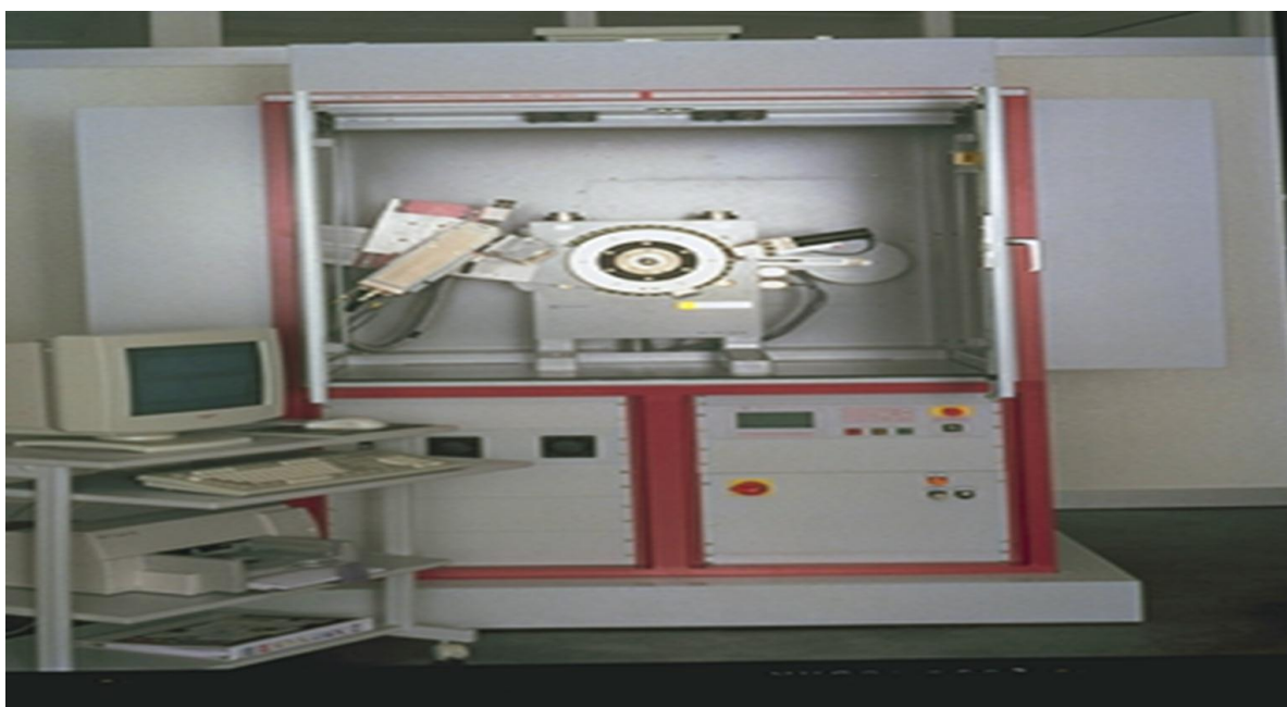
Figure 3-2: Schematic of Seifert 3003TT X-ray Diffractometer.
