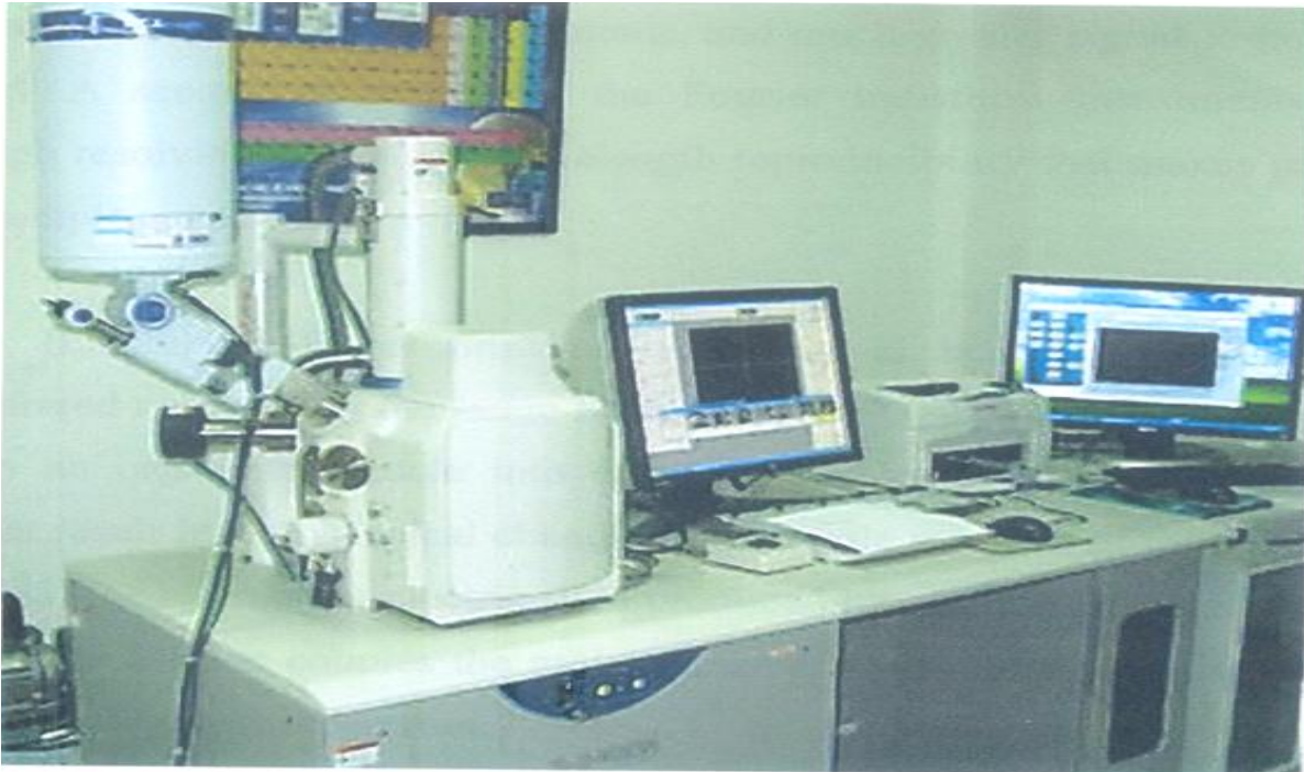
Figure 3-3: Schematic instrument of Scanning Electron Microscope.
