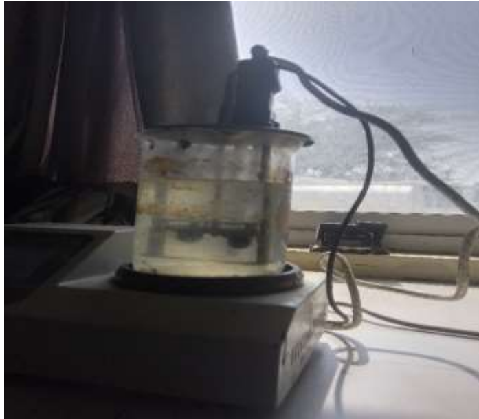
Figure 3. 10 Softening point test of bitumen
