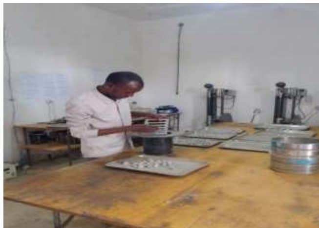
Figure 3.5 Flakiness index test
