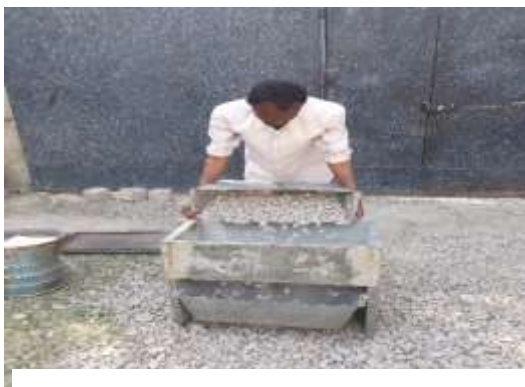
Figure 3. 2 a) Aggregate preparation b) Aggregate gradation
