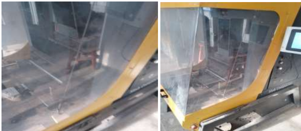
Figure 3. 19 a) Slab compactor Machine b) Slab compactor in motion
