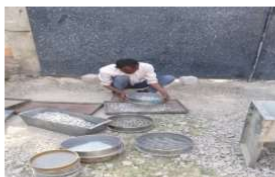
Figure 3. 2 a) Aggregate preparation b) Aggregate gradation
