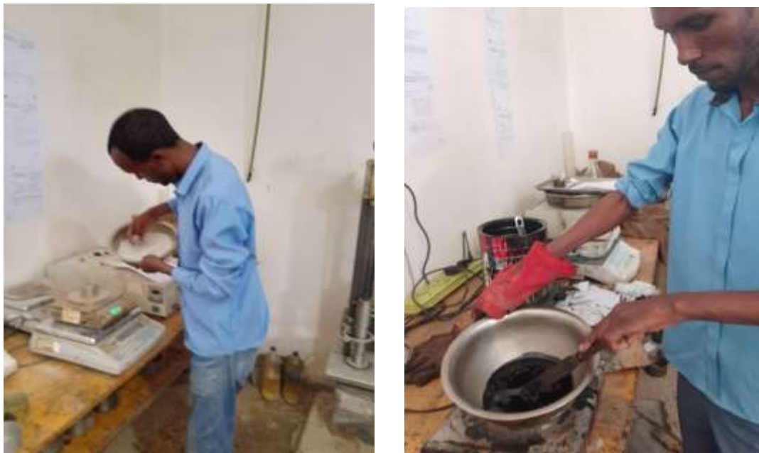
Figure 3. 25 Mixing of bitumen with shredded plastic in wet process
