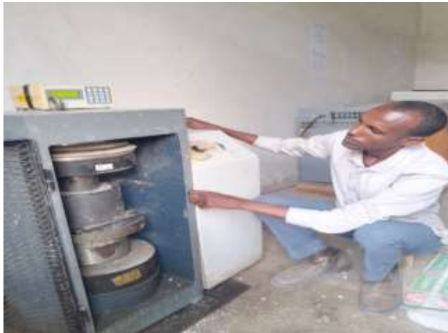
Figure 3. 4 Aggregate crushing value reading
