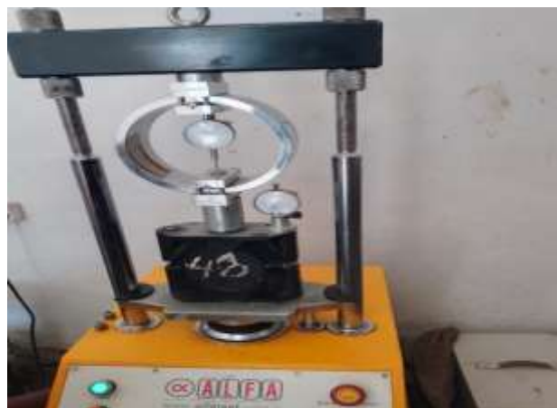
Figure 3.16 Marshall Stability and flow test for conventional mix
