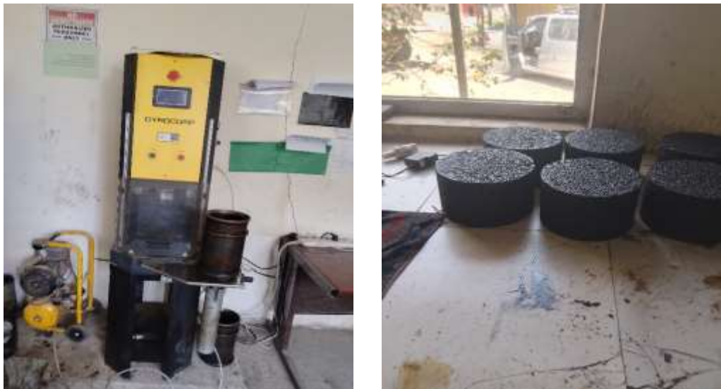
Figure 3. 22 a) Gyratory compaction b) Compacted specimen
