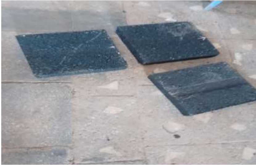
Figure 3. 21 Slab specimen after wheel tracking test
