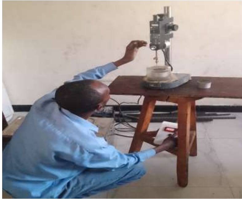
Figure 3. 9 Penetration test for bitumen
