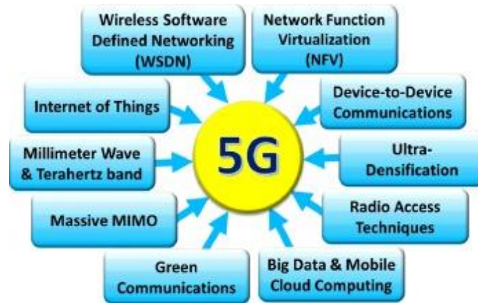
Figure 2.3 The 10 key enabling technologies for 5G (Akyildiz et al., 2016)
