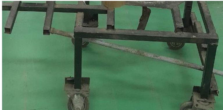
Figure 5.3 Fabricated stand of gasifier
