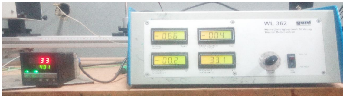
Figure A:10 Calibration setup of thermocouples with calibrator
