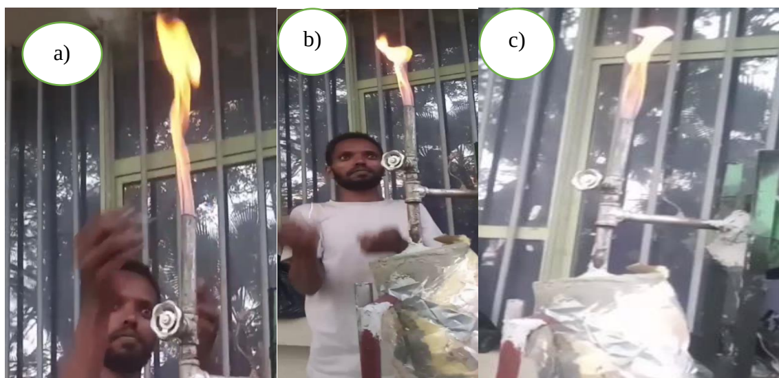
Figure 6.8 Comparison of flame intensity, (a) for corn cob ø10 mm pellet, (b) for corn cob ø20 mm pellet, and (c) for wheat straw ø10 mm pellets
