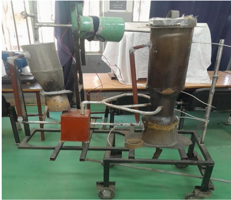
Figure 5.1 Fabricated different reaction zone of throat updraft gasifier
