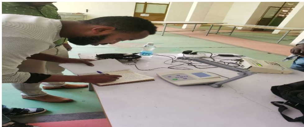
Figure 3.4. Analysis of ph and electrical conductivity
