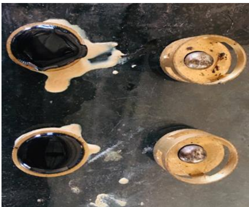
Figure 3.11 Sample preparation by ring ball and Softening point test
