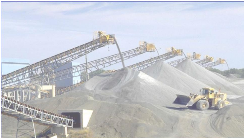
Figure 3.2 Aggregate production and Stockpile.
