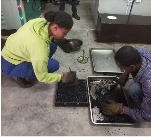
Figure 3.19 Sample preparation for rutting
