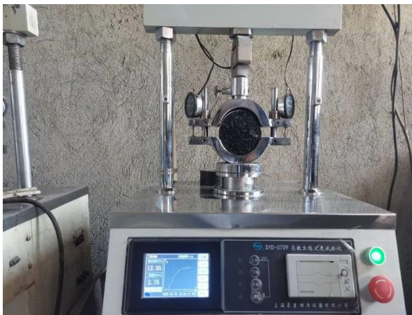
Figure 3.17 Stability & Flow Test.
