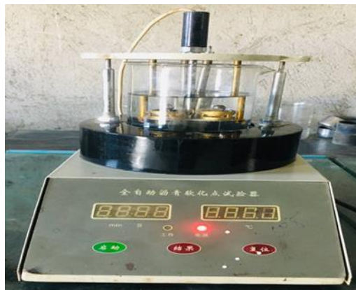
Figure 3.11 Sample preparation by ring ball and Softening point test
