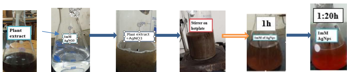
Figure 4: Synthesis silver nano particles using aqueous leaf extract of V. sinaiticum
