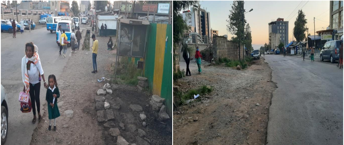
Figure 4. 74: Absence of sidewalk from Medhanialem Adebabayi to Mesalemiya in Addis Ketema Sub-Sub city
