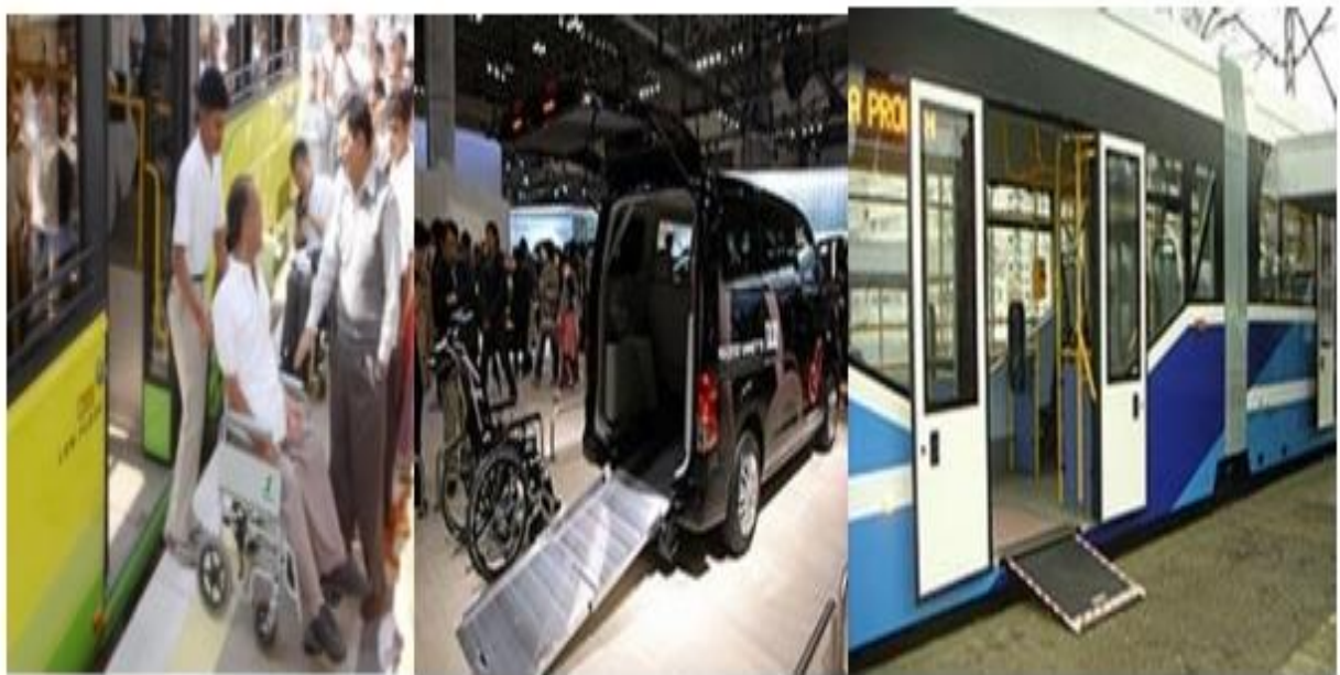
Figure 2.4: Low floor vehicle, minibus with a rear ramp and access by a ramp in the program.
