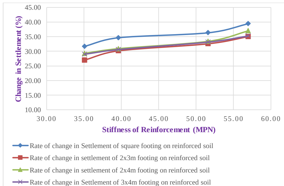
Figure 4.7: Effects of tensile modulus of reinforcement on the settlement of square and rectangular footing
