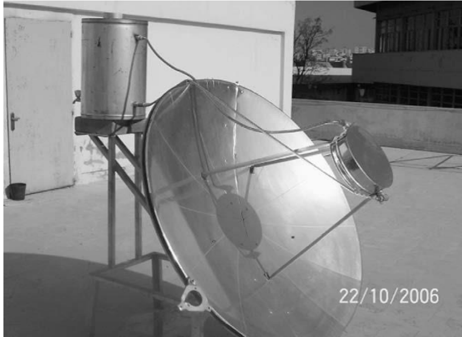
Figure 2.3 The device in the water heating mode (Badran et al., 2010).
