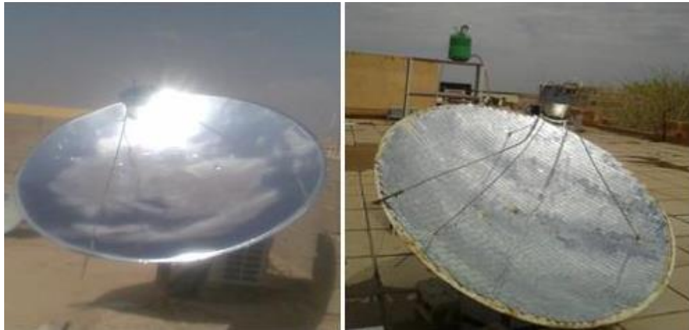
Figure 2.5 Parabolic dish concentrator for water heating purpose (Yaseen et al. , 2018).
