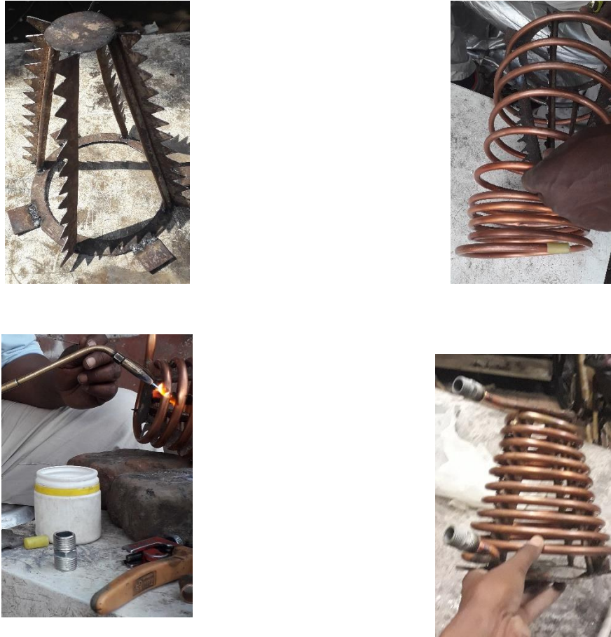
Figure 6.3 Manufacturing process of conical cavity receiver, a) Structure of cone b) Rolling copper tube on structure c) Gas welding conical structure with copper tube d) Conical tube receiver.
