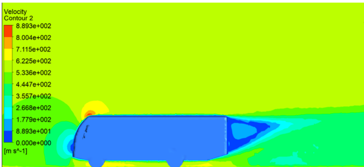
Figure 5. 25 velocity contour of modified bus at 100km/h
