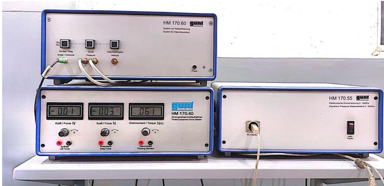
Figure 4. 21 Zeroing the measuring amplifier
