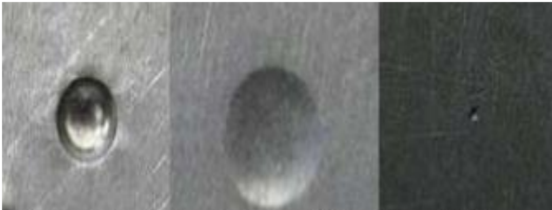
Figure 2.5 The indentation of Rockwell, Brinell, Vickers hardness test respectively [63]
