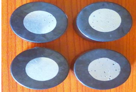
Figure 3.12 Microstructure test specimens
