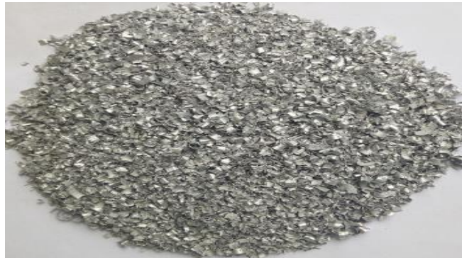
Figure 3.1. Aluminum (AA6063) alloy powders
