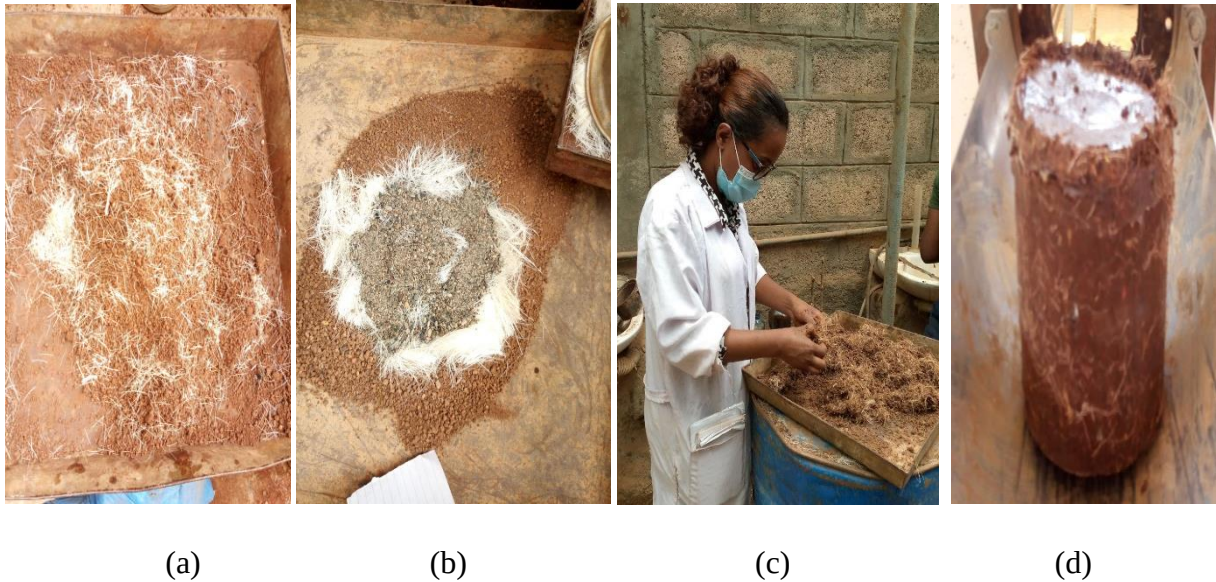
Figure 3.5. Photographic view of (a) dry mix of clay soil and Katcha fiber; (b) preparation of soil-fiber-sand mix, (c) mix preparation for compaction test (d) remold soil sample of reinforced soil.
