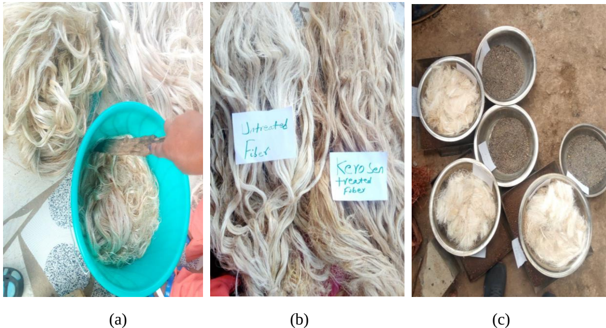
Figure 3.3. Photographic view of (a) Katcha fiber soaking; (b) Air dried Kerosene soaked Katcha fiber and (c) 35 mm length Katcha fiber and Sand.
