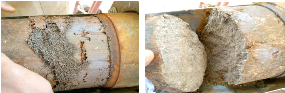
Figure 3.4. Photographic view of one of the position of sandy layer in compaction mould.
