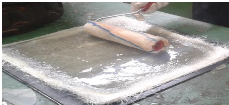
Figure 3.7. Removing of air using roller
