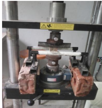
Figure 3.12. Specimen under bending test
