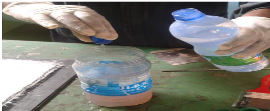
Figure 3.6. Mixing of epoxy with hardener
