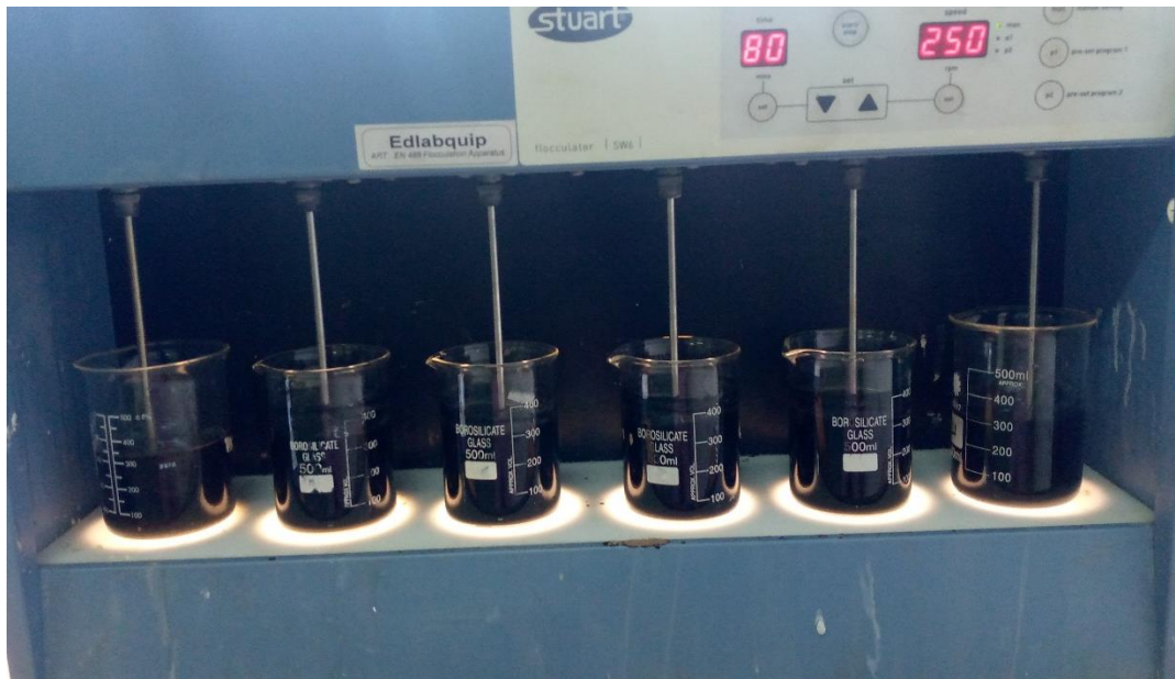
Figure 3.5: Batch adsorption experiment to test adsorption parameters
