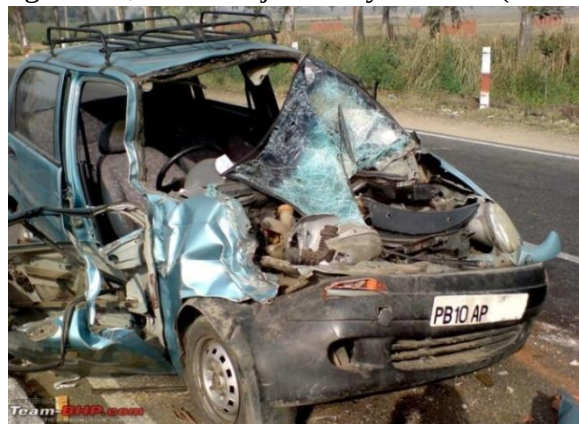
Figure 1.2. Vehicle damage after under run accident (Cottingham 2022)
