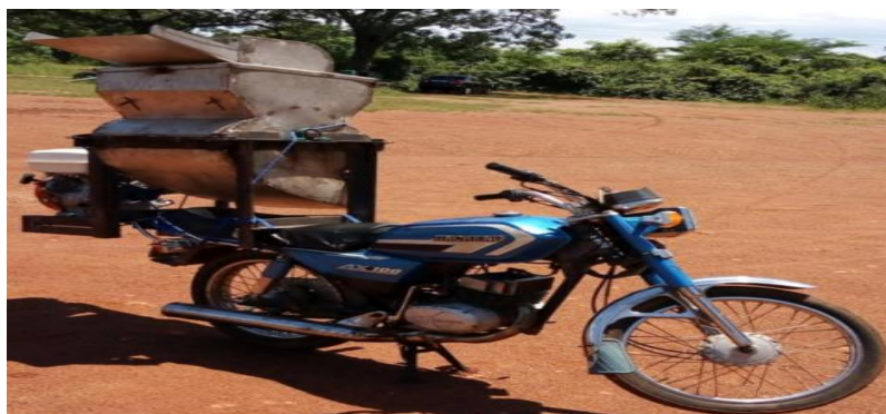
Figure 13. Modified NCAM grater. Source: Ogunjirin et al. (2020)
