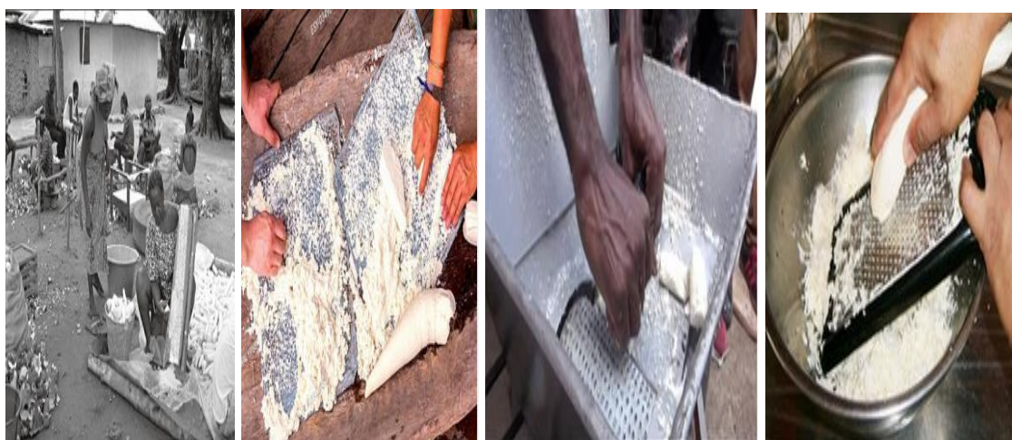
Figure 8. Perforated metal plate grater. Source: Joseph (2017)
