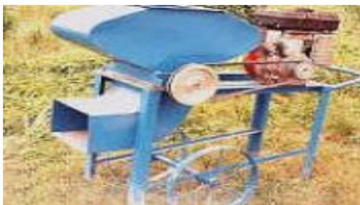
Figure 14. Stationary or mobile cassava grater. Source: Apodi et al. (2018)
